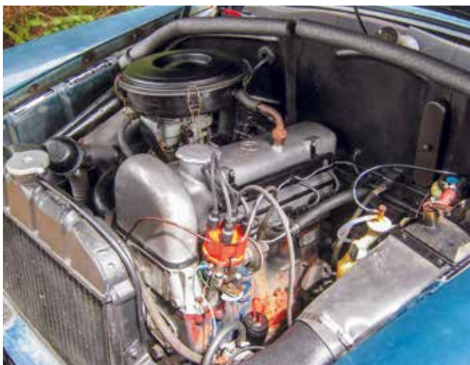
TOP: Departure, 10 a.m. on September 23, 2013. Tom holds the “Good Luck” card from fellow volunteers at the New England Air Museum. ABOVE LEFT: The 90-horsepower 4-cylinder M-121 engine, cleaned up, tuned, and ready to go. ABOVE RIGHT: A stop in Appleton, Wisconsin, to visit former student Paul Wilke, his wife Jill, and sons Tom and Matt.
