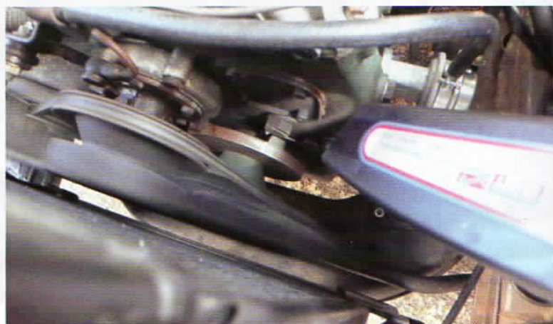
Using a strobe light to check the timing.
