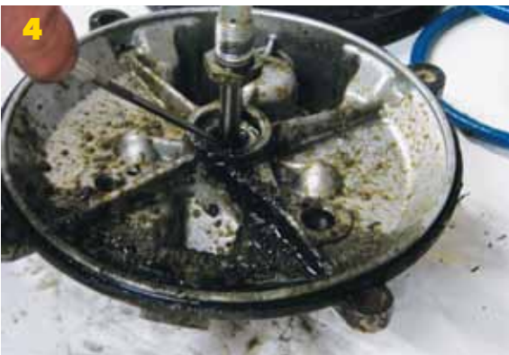
1. Typical brake booster upon arrival 2. The disassembled booster 3. Note the brake fluid that leaked into the vacuum chamber. This will result in losing brake fluid and finding its way into the engine. Result, low brake fluid in the reservoir and
