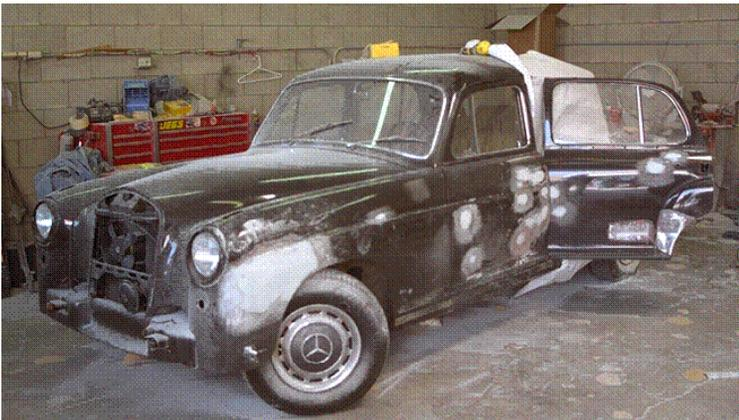
These pictures were taken during the exterior restoration. The work included body repairs, grill refinishing, painting and clearcoat. The color is dark green, as close to the original DB259, (non-metallic) Forest Green as we could get, using the chips available. Paint was done in Ditzler Durethane, by Rainbow Painting in San Luis Obispo, CA.
