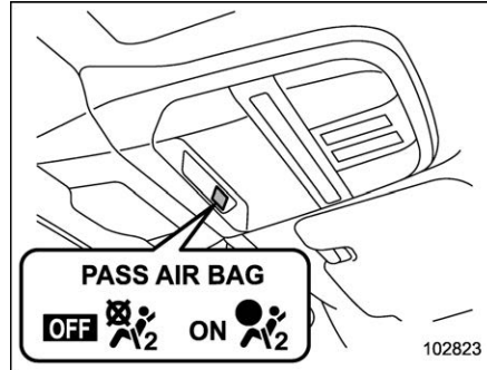
ON : Front passenger's frontal airbag ON indicator light OFF : Front passenger's frontal airbag OFF indicator light
