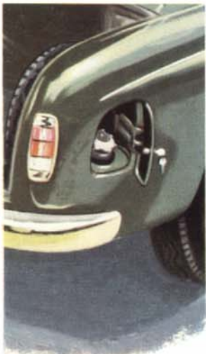
A lockable lid in the right rear fender skirt protects the gas tank filler from unauthorized interference.
