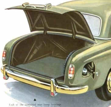
Each of the combined rear lamp housings comprises a tail light, a stop light, a blink light for the direction indicator, and a parking light. In addition to those there is a powerful bulb in the left lamp which lights automatically when the car is driven backwards. The current-saving front and rear parking lights can be turned on either on the right, or on the left, or on both sides.
