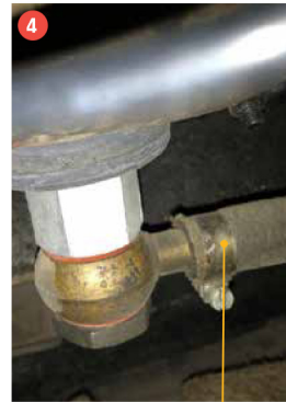
Vacuum Hose to Booster As seen from under dash - disconnect hose
