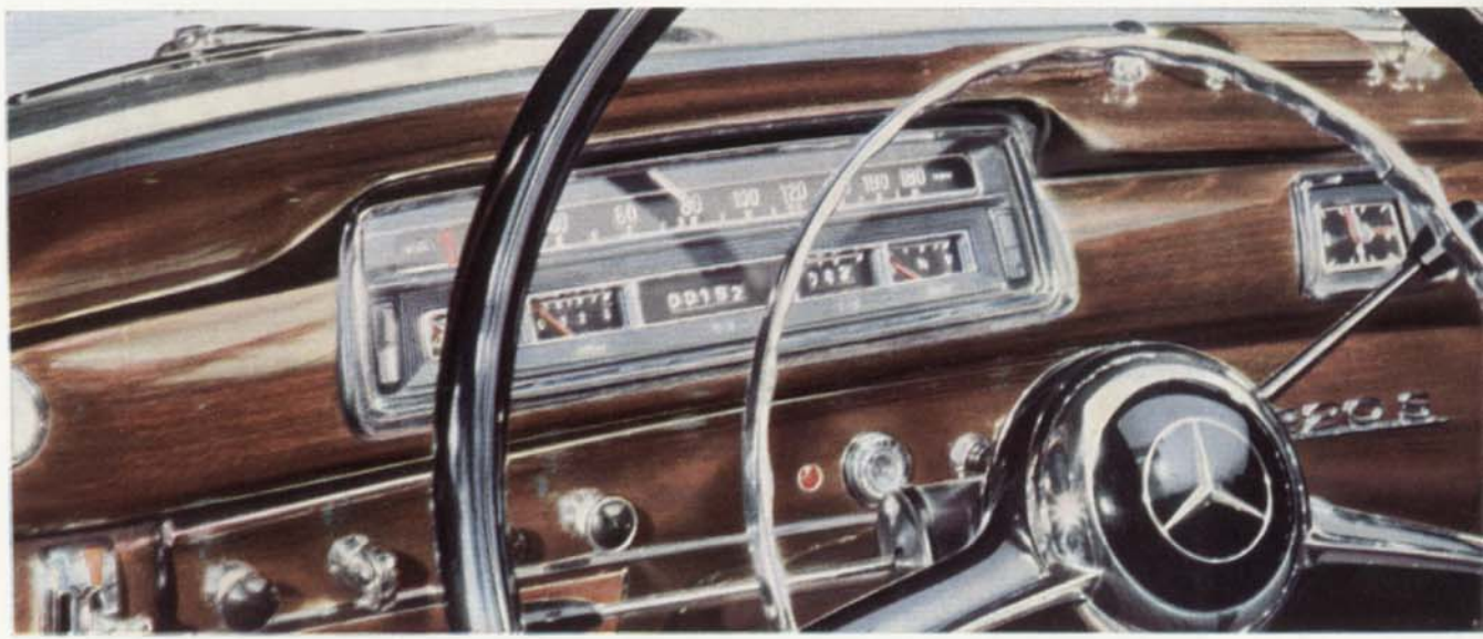
At a slightly higher cost, the 220 S is equipped with a flawless hydraulic automatic Daimler-Benz-clutch. It does away with the clutch pedal and further simplifies driving. A special brochure explains its advantages and function.
