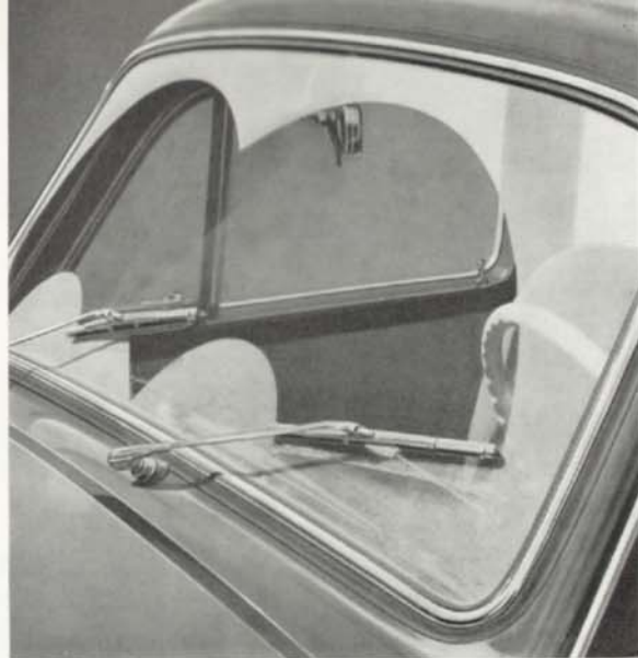
When it rains, the windshield wipers sweep a large unbroken field of vision across the windshield. This is an important driving aid for the driver. They are controlled by a two-speed switch on the dashboard.
