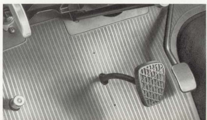
At a slightly higher cost, the 220 S is equipped with a flawless hydraulic automatic Daimler-Benz-clutch. It does away with the clutch pedal and further simplifies driving. A special brochure explains its advantages and function.
