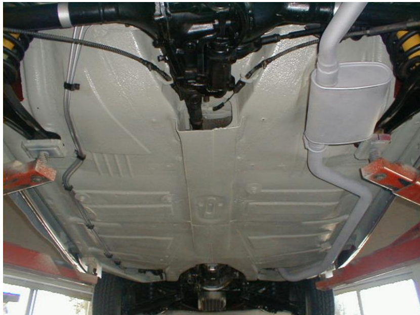
Second photo: Underbody of a restored 190SL with a close match to DB 169.
