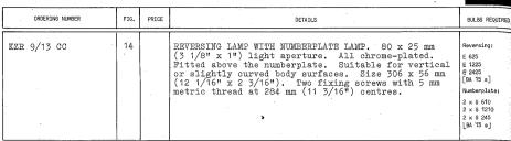
The use of Speedo-Mounted Reversing Lamp Switches (see under "Switches") enables these lamps to automatically switched on when the vehicle begins to reverse.
